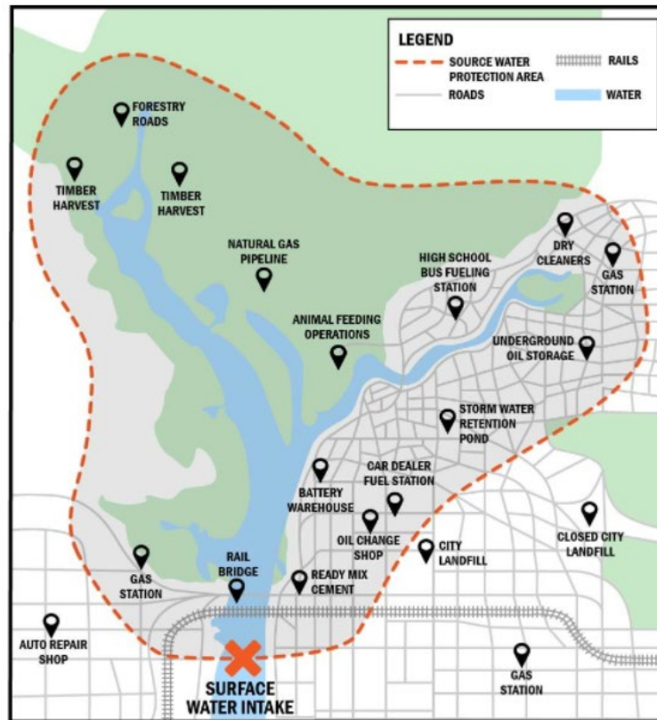
Inventory Potential Sources of Contamination
