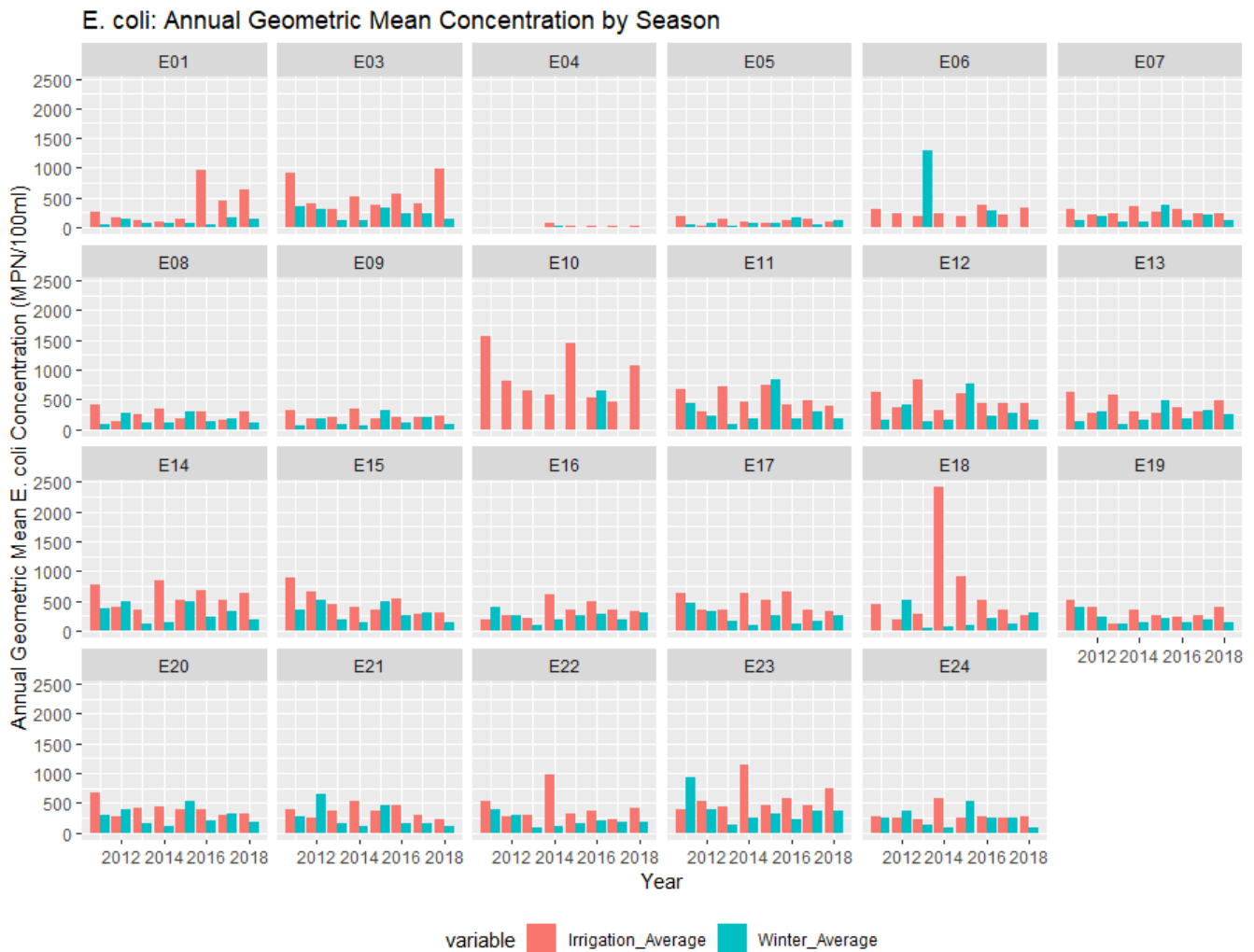
Figure 7. Annual geometric mean E. coli concentration by season. Irrigation season (red columns) defined as samples taken April 15 th – October 15 th ; winter season (blue columns) defined as samples taken October 16 th – April 14 th .
