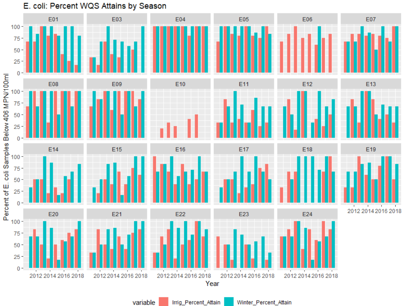
Figure 6. Percent of E. coli samples that attain the water quality standard per year by season.
